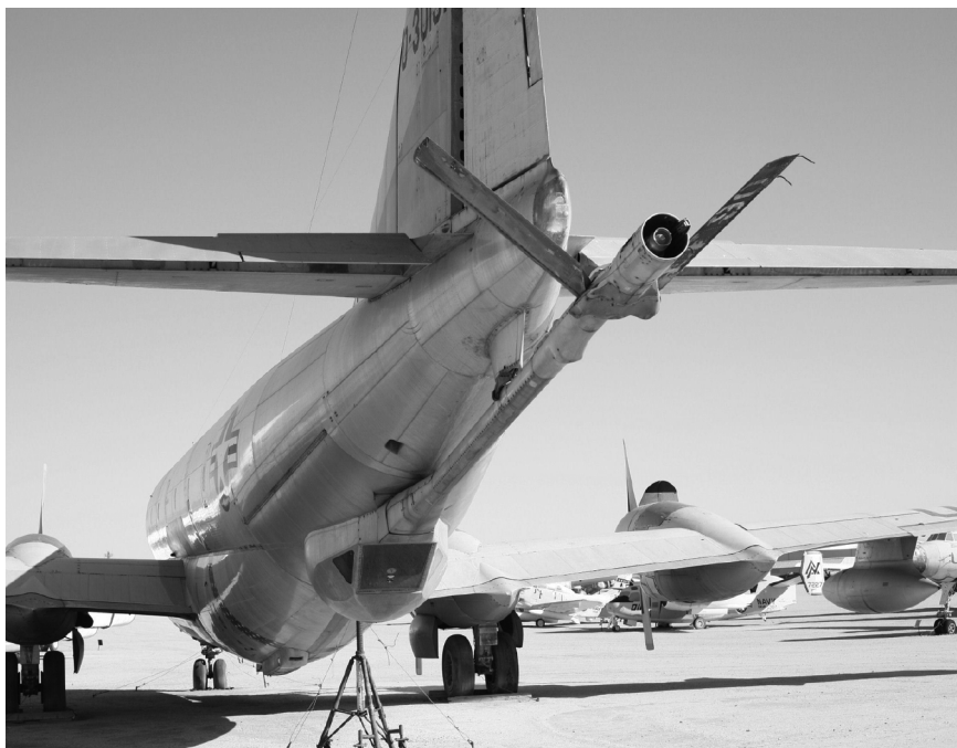
Figure 3. Underneath the KC-97 is also a refueling boom (shown here in stowed position). When down, the boom is at an angle consistent with the sixty degrees an eyewitness reported (specifically sixty-four degrees, according to the flight manual). The sequencing lights would reflect onto the boom, which would flutter “like a floating leaf” when not controlled by the boom operator (note its small wings). [Photos by James McGaha]
