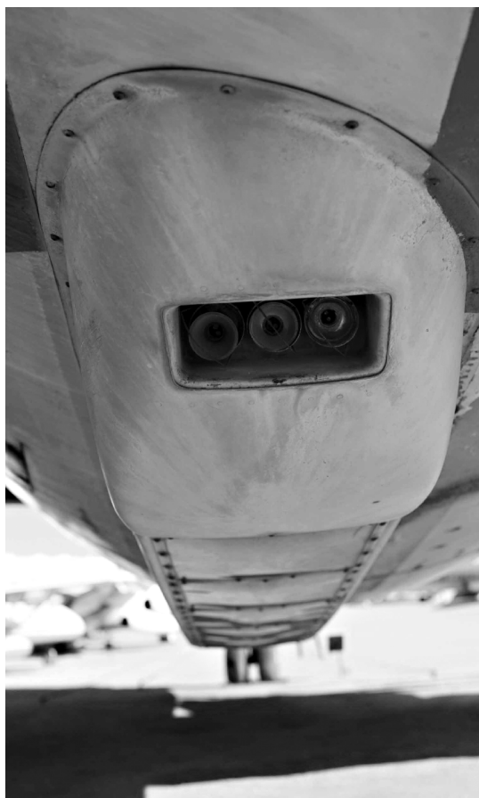
Figure 2. On the underbelly of the KC-97 are [closest to the camera] a set of three high-intensity lights and [farther from the viewer] the five red panels of sequencing lights. (These were described by eye-witnesses as “five bright red lights” that “flashed on one at a time,” specifically “pulsating: one, two, three, four, five, four, three, two, one.”)
